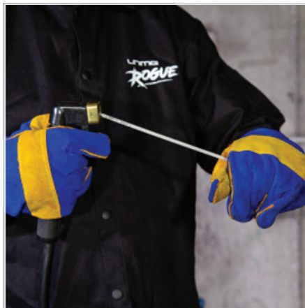
(4) Place the electrode into the electrode holder and clamp tight.
